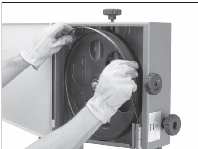
Figure 36. Placing blade on the wheels.
